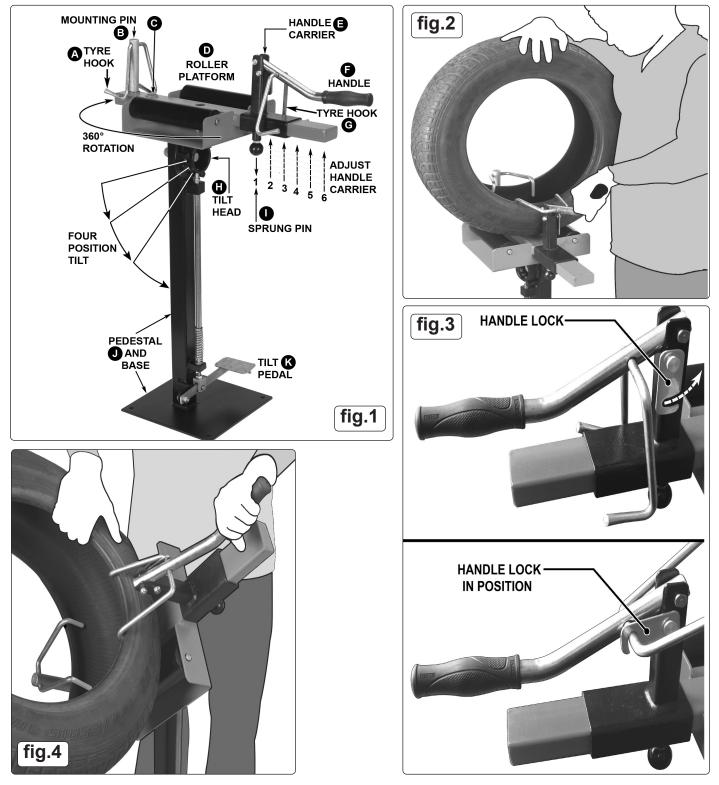
5.4 Push the handle over centre into the down position to stretch the tyre. On the side of the Handle Carrier upright is a locking plate. Rotate the handle locking plate around so that the slot in it drops over the tyre hook (G) to prevent the handle moving upwards. See fig.3.
